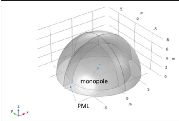
**Figure 5.** Radiation of a monopole in a half-space.
