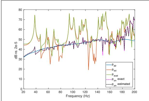
**Figure 8.** Pressure with and without control on microphone MicD 1 for the test source SourceID 30.
