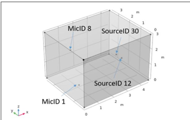
**Figure 6.** Source (number 12, 30) and microphone (number 1, 8) identification positions.
