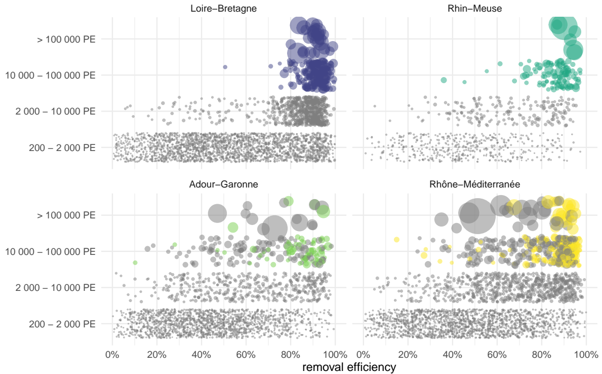
Figure 3: Individual WWTP P removal efficiencies, averaged over 2015-2020, in 4 of the French water agencies basins. Each dot is a WWTP, size is proportional to nominal capacity, expressed in population equivalent (PE). Dots are highlighted if the WWTP must reach minimal performances due to P sensitive area classification (see Figure 2a and text).
