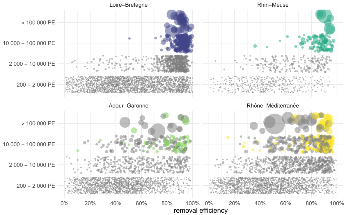
Figure 3: Individual WWTP P removal efficiencies, averaged over 2015-2020, in 4 of the French water agencies basins. Each dot is a WWTP, size is proportional to nominal capacity, expressed in population equivalent (PE). Dots are highlighted if the WWTP must reach minimal performances due to P sensitive area classification (see Figure 2a and text).
