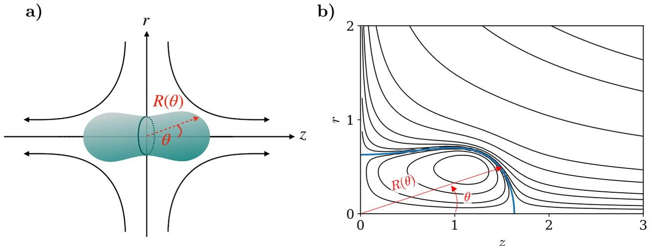
FIG. 1. a) Scheme of a bubble at the center of a uni-axial straining flow. ( $Oz$ ) is the axis of symmetry. Arrows show typical streamlines in the absence of bubble. b) Enlargement around a bubble experiencing its maximum deformation at  $Re = 400$  and  $We = 7.3 \approx We_c(Re = 400)$ . The blue line denotes the bubble interface, black lines, isocontours of the stream function.
