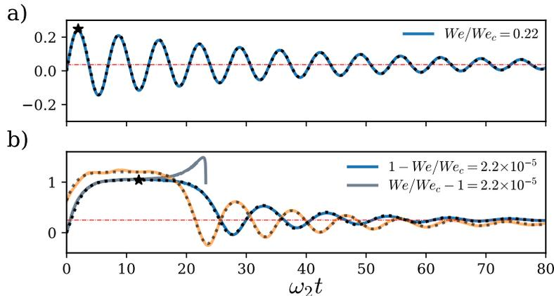
FIG. 3. a) & b) Several typical temporal evolution of  $x$  at  $Re = 400$ . Simulation data are in color, the model (4) is superimposed (black dotted line). a) An initially spherical bubble at low  $We$ . b) Three evolutions close to  $We_c(a_0)$ , for a stable sphere (blue line), an unstable sphere (grey line) and a stable ellipsoid (orange line,  $a_0 = 0.8$ ).
