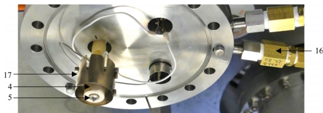
Fig. 4. Furnace and indenter installed on the cooling flange.
