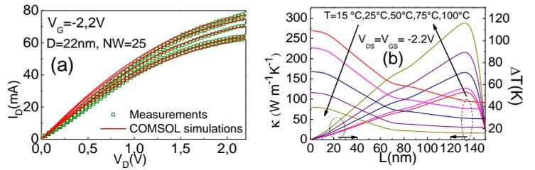
Fig. 2 (a)  $I_D$ - $V_D$  of a p-type VNWFET comparing COMSOL simulations with DC temperature measurements. (b) Thermal conductivity and internal device temperature under different temperature condition.
