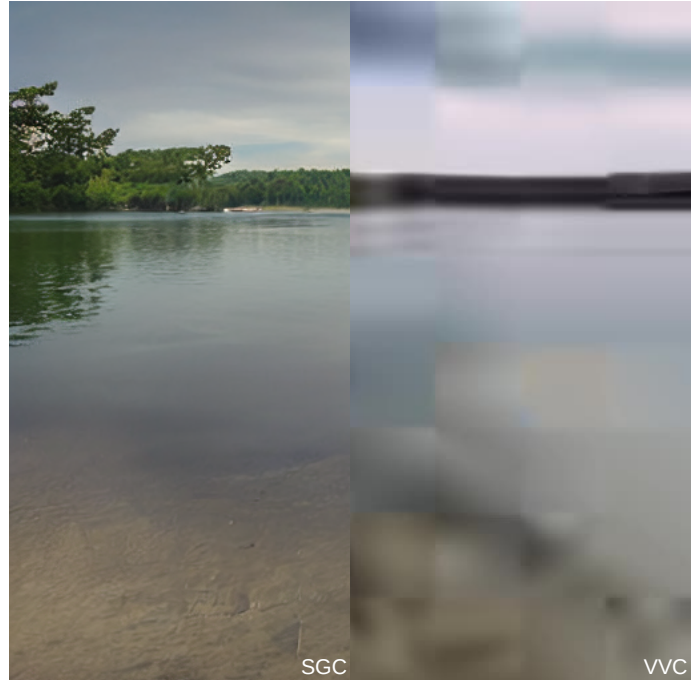
Fig. 1. Illustration of the perception-distortion tradeoff. Pixel (VVC) and semantic fidelity (SGC) compression methods side-by-side at extremely low bitrates (0.022 bpp). VVC which optimizes the MSE loses the semantic, while our approach manages to show semantic and visual quality at the same time.
