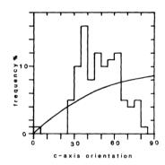
**Figure 10.** Texture obtained after 9% of octahedral tension strain (about 13% axial strain) performed at  $-3^{\circ}C$  with an octahedral stress of 0.4 *MPa*. The star ★ in the centre of the pole figure shows the direction of the tension axis. From Jacka et al. 1984 [27].
