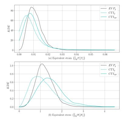
**Figure 6.** Kernel Density Estimation of the Von Mises equivalent strain (a) and stress (b) fields simulated with CraFT-EVP (EVP, black line) and  $R^3$ iCe (CTI, cyan line). The dashed lines show results obtained for simulations where grains are defined by multiple mesh elements (*grains* microstructure) (figure 4 *a-b*). The full line shows a  $R^3$ iCe simulation where a single orientation is attributed per element (figure 4 *c*)
