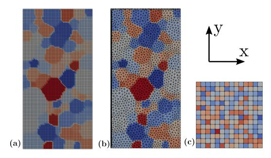
**Figure 4.** Microstructure generated via a grain growth using Neper meshed for (a) CraFT-EVP microstructure with 265302 grid points (b) R<sup>3</sup>iCe with 262688 tetrahedral elements. (c) Simplified microstructure in which orientations are defined at the element scale with hexahedral mesh of 2740 elements.
