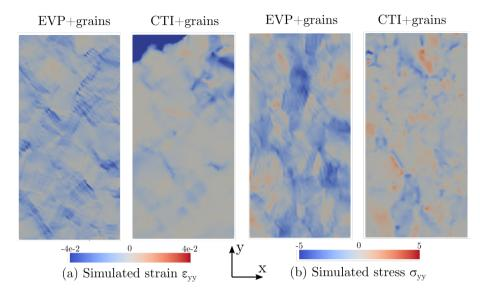
**Figure 5.** Comparison of predicted (a) strain  $(\varepsilon_{yy})$  (b) stress  $(\sigma_{yy} = S_{yy} + p)$  fields for the "grain" microstructure using CraFT-EVP and R<sup>3</sup>iCe.
