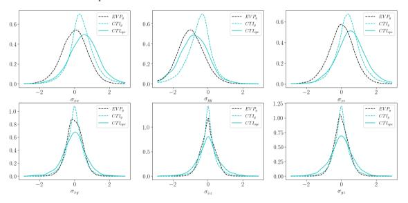
**Figure 16.** Kernel Density Estimation of all components of the stress tensor predicted by an elasto-viscoplastic (EVP) simulation using CraFT and the Continous Transverse Isotropic (CTI) using R<sup>3</sup>iCe after 0.01 macroscopic strain. The dashed lines show results for simulations where grains are well discretized. The full line shows result for the simulation with one orientation per element.
