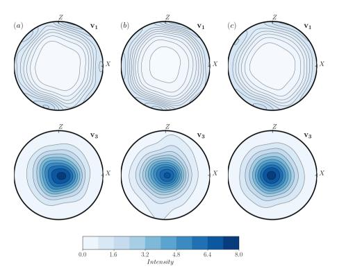
**Figure 7.** Distributions of the principal stress tensor directions  $\mathbf{v_1}$  and  $\mathbf{v_3}$  for uniaxial compression on (a) CraFT-EVP simulation (b)  $R^3$ iCe simulation with grains (c)  $R^3$ iCe simulation with one orientation per mesh element.
