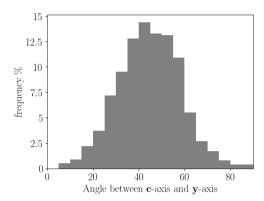
**Figure 12.** Distribution of the angle between the **c**-axis and the **y**-axis (tension axis) corresponding to the pole figure (*ii*) in figure 11d.
