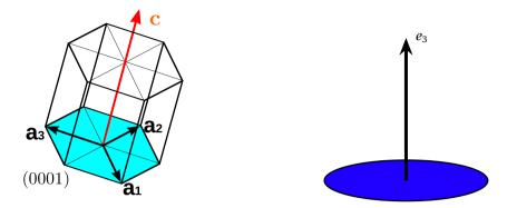
**Figure 1.** The transverse isotropic geometry is fully described by one direction,  $e_3$ , that defines the plane of isotropy. For an ice single crystal, this direction corresponds to that of the **c**-axis (i.e. the normal to the basal (0001) plane).
