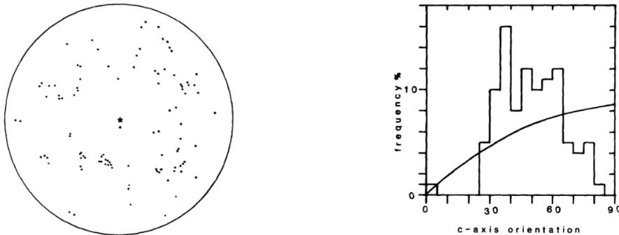
**Figure 10.** Texture obtained after 9% of octahedral tension strain (about 13% axial strain) performed at  $-3^\circ\text{C}$  with an octahedral stress of  $0.4\text{ MPa}$ . The star  $\star$  in the centre of the pole figure shows the direction of the tension axis. From Jacka et al. 1984 [27].
