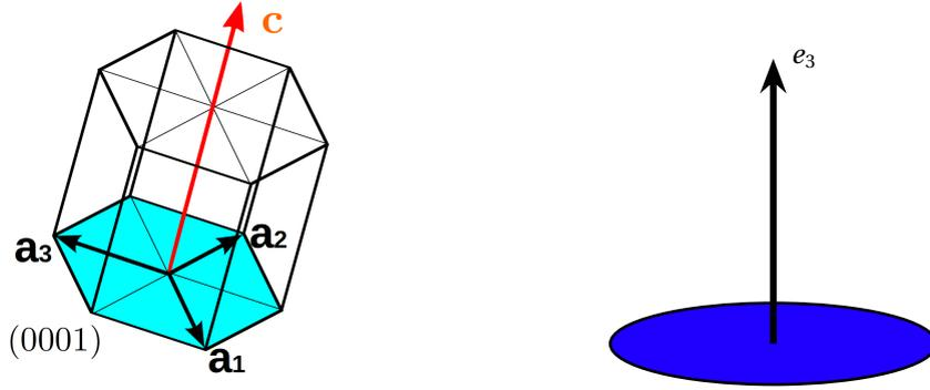
**Figure 1.** The transverse isotropic geometry is fully described by one direction,  $e_3$ , that defines the plane of isotropy. For an ice single crystal, this direction corresponds to that of the  $c$ -axis (i.e. the normal to the basal (0001) plane).
