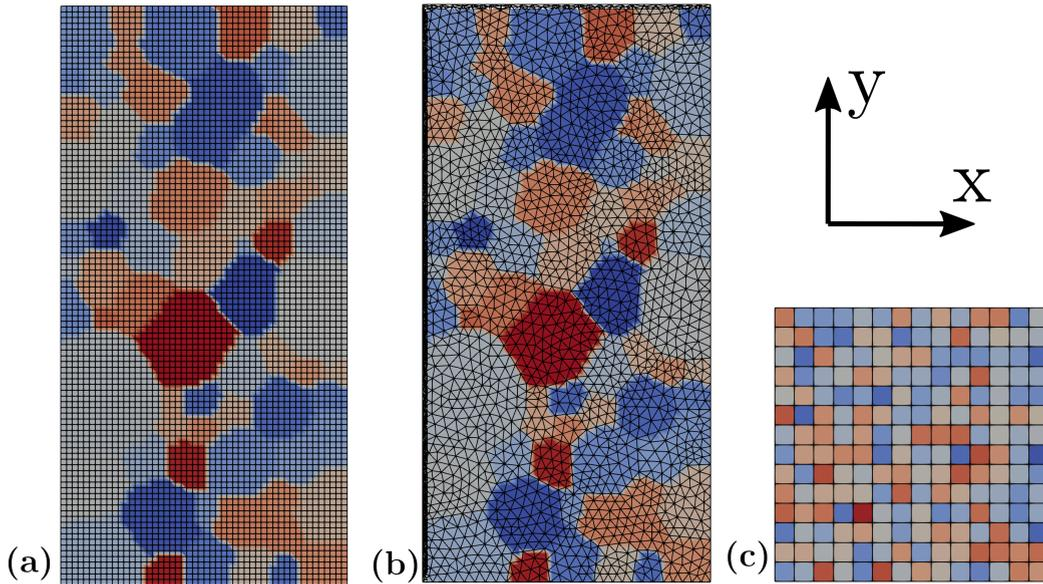
**Figure 4.** Microstructure generated via a grain growth using Neper meshed for (a) CraFT-EVP microstructure with 265302 grid points (b)  $R^3iCe$  with 262688 tetrahedral elements. (c) Simplified microstructure in which orientations are defined at the element scale with hexahedral mesh of 2740 elements.
