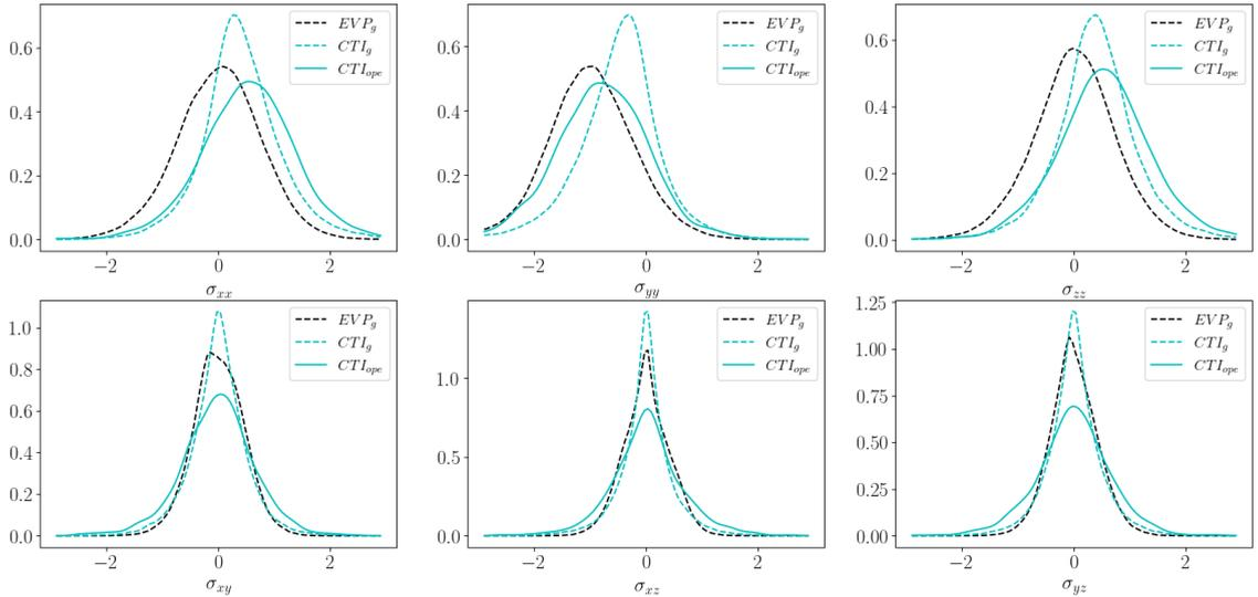
**Figure 16.** Kernel Density Estimation of all components of the stress tensor predicted by an elasto-viscoplastic (EVP) simulation using CraFT and the Continuous Transverse Isotropic (CTI) using R<sup>3</sup>iCe after 0.01 macroscopic strain. The dashed lines show results for simulations where grains are well discretized. The full line shows result for the simulation with one orientation per element.
