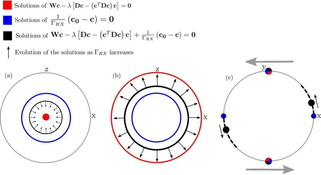
**Figure 2.** Pole figure schematic representation of the stable orientations for the evolution equation (eq. 22) for various stress configurations  $\mathbf{S}$ : (a) uniaxial compression along  $\mathbf{y}$ , (b) uniaxial tension along  $\mathbf{y}$  and (c) simple shear in the  $xOz$  plane,  $\frac{\partial u_x}{\partial y} < 0$  (upper hemisphere).
