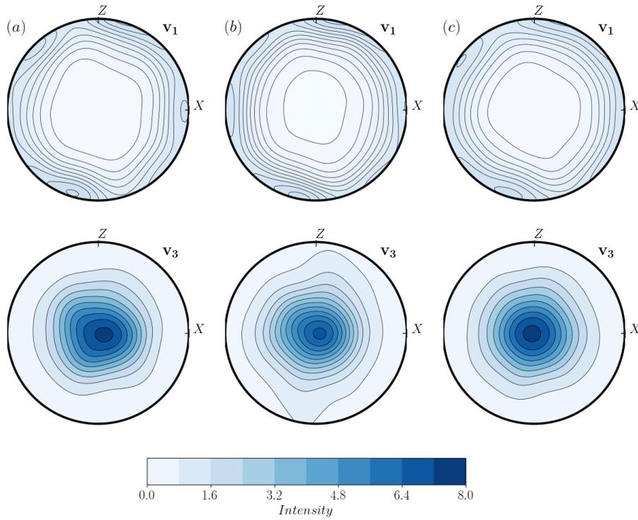
**Figure 7.** Distributions of the principal stress tensor directions  $\mathbf{v}_1$  and  $\mathbf{v}_3$  for uniaxial compression on (a) CraFT-EVP simulation (b) R<sup>3</sup>iCe simulation with grains (c) R<sup>3</sup>iCe simulation with one orientation per mesh element.
