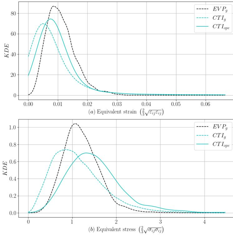
**Figure 6.** Kernel Density Estimation of the Von Mises equivalent strain (a) and stress (b) fields simulated with CraFT-EVP (EVP, black line) and R<sup>3</sup>iCe (CTI, cyan line). The dashed lines show results obtained for simulations where grains are defined by multiple mesh elements (*grains* microstructure) (figure 4 *a-b*). The full line shows a R<sup>3</sup>iCe simulation where a single orientation is attributed per element (figure 4 *c*)
