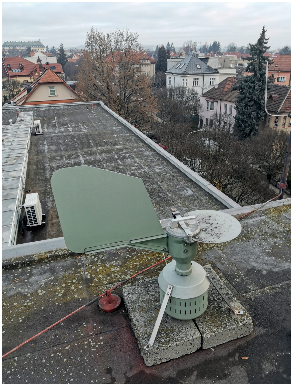
Figure 1. 7-day volumetric air sampler (Burkard Manufacturing Co Ltd, Hertfordshire, UK) in Brno (Czechia) installed on the roof of the University hospital, 15 m above ground to ensure landscape-scale monitoring. Photo credit for Aneta Lukačevičová.
