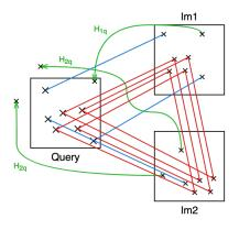
Figure 3: Query image set of keypoints with solid points in red, unsolid points in blue and reprojected ones in green
