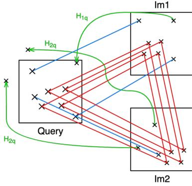
**Figure 3: Query image set of keypoints with solid points in red, unsolid points in blue and projected ones in green**
