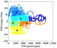
Fig. 2: Clusters and centroids obtained by k-means applied to a WLTC
