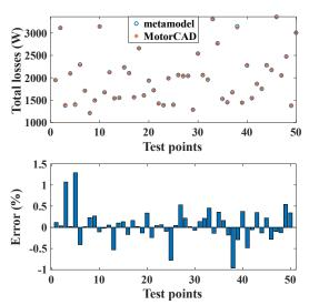
Fig. 10: Evaluation of the precision of losses metamodel
