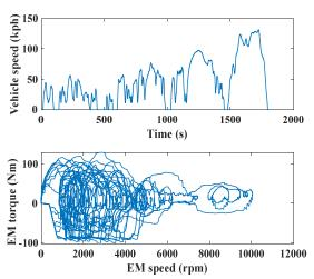
Fig. 1: Electric machine torque and speed for WLTC cycle
