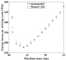
Fig. 11: Optimization results and comparison with MotorCAD calculations
