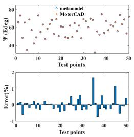
Fig. 9: Evaluation of the precision of phase advance metamodel
