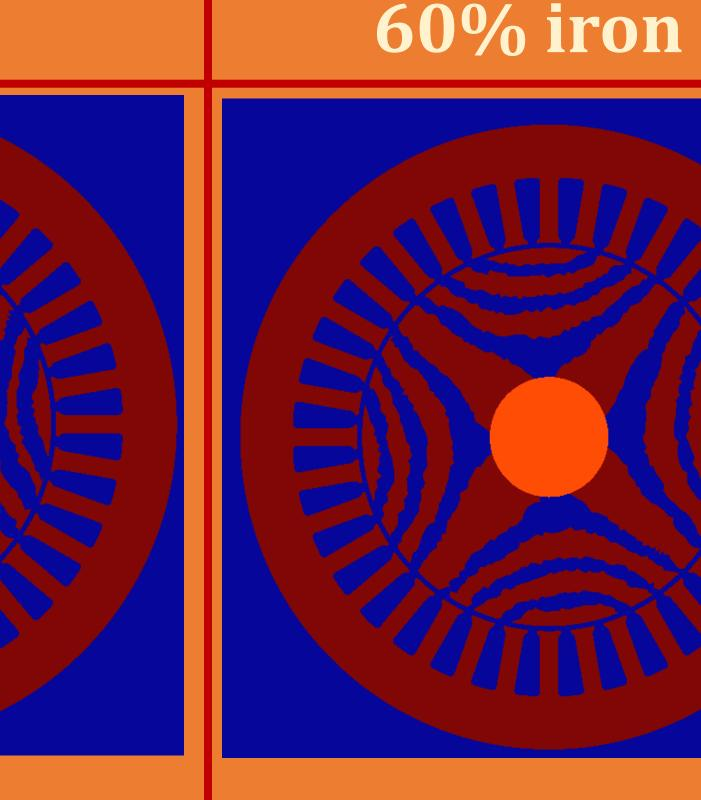
The number of elements in the rotor is <u>8642</u>. The convergence is different for each volume. For 60% of iron, the number of iteration is equal to 1000, and the total time is <u>12min</u>
