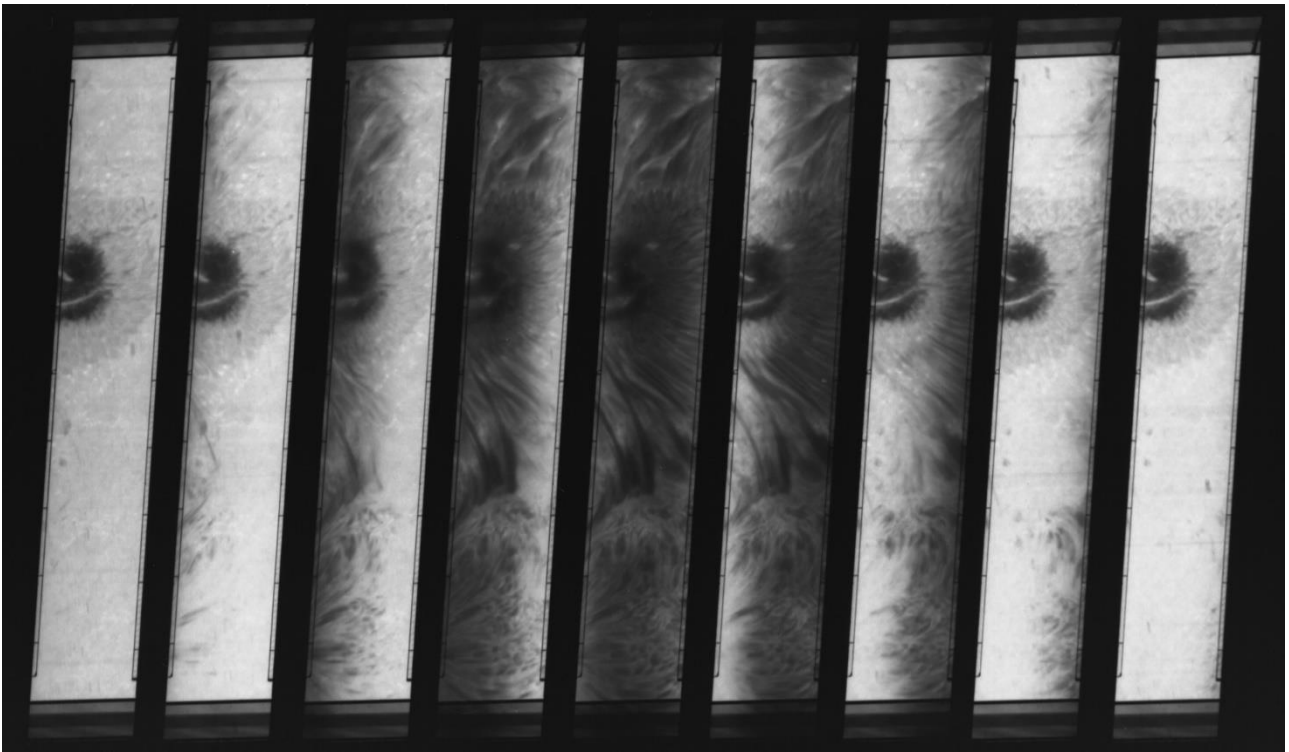
Figure 4: the MSDP of the Vacuum Tower Telescope (9 channels, H \alpha line, sunspot and active region).
