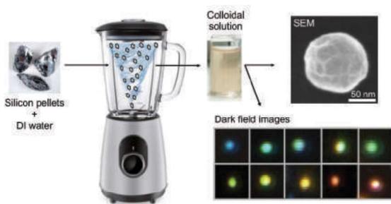
Figure 1: Fabrication of Silicon Mie resonator using a blender. The various diameters give a full range color spectrum scattering.
