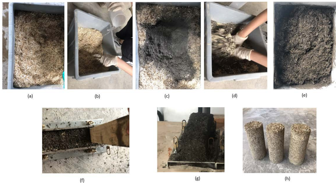
Figure 1 Process of hemp concrete design for bending specimens; (a): dropping of hemp shives, (b): wetting of hemp shives, (c): put on CSA cement, (d): hand mixing of hemp shives with water and cement, (e): status of the resulting mixture, (f): compaction loads on hemp concrete inside the molds, (g): demolded hemp concrete in the case of the parallelepiped molds, (h): demolded hemp concrete in the case of the cylindrical specimens.
