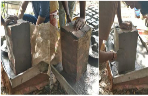
Figure 6 : Application de FRCM en confinement [90]
