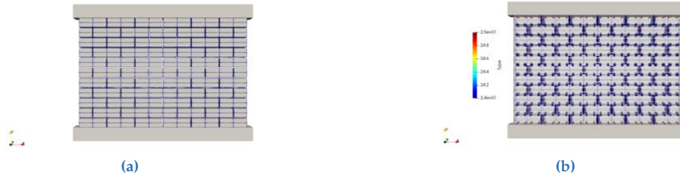
FIGURE 7. Numerical model of the wall : (a) wall mesh (b) contact points.
