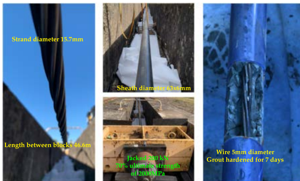
FIGURE 4. Photos of the experimental bench at various step of the experiment set up
