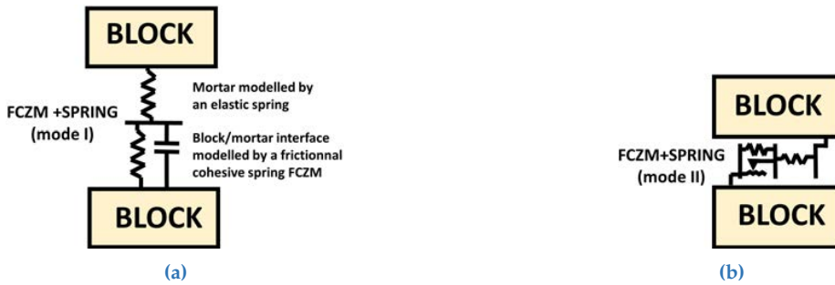
FIGURE 5. Rheological model of the proposed contact law : (a) in mode I (b) in mode II.
