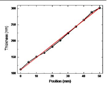
**Fig. 6** | **Calibration of the wedge deposition thickness.** Variation of the thickness of a thick Cu wedge as a function of position.
