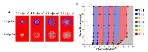
Fig. 3 | Single-pulse reversal in  $Tb_{32}Co_{68}(4 \text{ nm})/Co(1.52 \text{ nm})/Tb_{32}Co_{68}(4 \text{ nm})$  trilayer. a Background subtracted images after first and second pulses with 50 fs laser pulse with different fluences. b State diagram which is plotted by pulse duration as a function of fluences.  $TF_1$  is the border for switching;  $TF_2$  is the border
