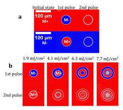
Fig. 1 | Single-pulse switching and state diagram for [Tb(1.31 nm)/Fe(1.89 nm)]<sub>4</sub> multilayer under zero applied field. M+ (respectively, M–) corresponds to magnetization pointing perpendicular to film plane, along +z (respectively –z) in red (respectively in blue). a Background subtracted images after each single pulse with 1.9 mJ/cm² laser pulse at 50 fs, starting from M+ or M- state. b Background
