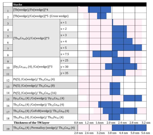
Light pink color shows the TM layer (including Co, Fe, CoFeB, Permalloy) thickness range that have been studied in this paper, while blue color shows the region of TM thickness where single-shot switching occurs in different stacks. Note that stack 1 is a double wedge sample in the same direction, while stack 2 is a cross-wedge sample. Numbers shown within the brackets are the layer thicknesses in nanometers.
