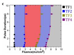
subtracted images after first single with 50 fs laser pulse of different fluence.  $\mathbf{c}$  State diagram of reversal pulse duration versus fluence.  $\mathsf{TF}_1$  is the border for switching;  $\mathsf{TF}_2$  is the border to two domains state (i.e., one ring);  $\mathsf{TF}_3$  is the border to three domains state (i.e., two rings);  $\mathsf{TF}_4$  is the border to multidomain state at the center (i.e., three rings). The dotted lines are guide for the eyes.
