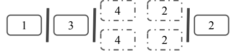
(c) Optimal schedule for P = 6 . Tasks in s_3 are duplicated to represent p_3 = 2 . Only P' = 5 is necessary for the optimal solution.
