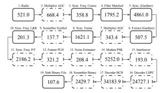
Fig. 2: Illustration of the DVB-S2 reception chain. Each box represents a task. Task names (adapted from [30]) and task weights (rounded values in  $\mu$ s) are given with each task. Solid (resp., dashed) lines represent stateful (resp. stateless) tasks.
