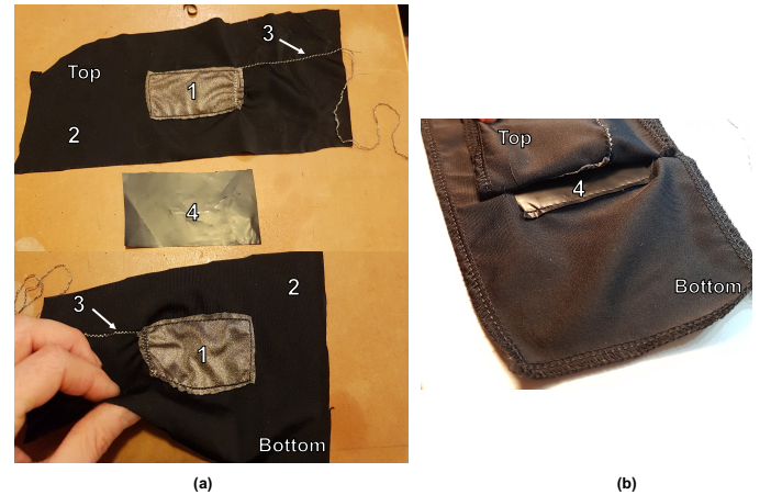
Fig. 5: Manufacturing of a piezoresistive sensor with electrodes made of conductive textile material: (a) The 5 layers of the sensor, where (1) is the conductive textile tape (0.55 mm), (2) the polyamide elastane fabric, (3) the conductor wire and (4) the piezoresistive layer (0.1 mm thick); (b) The sandwich structure before final closing.
