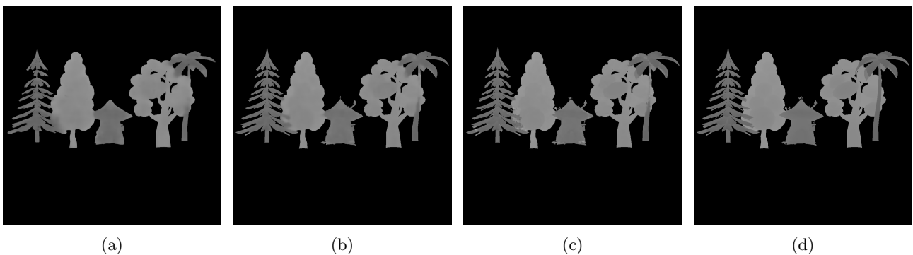
Figure 3: The intermediate results generated by the network after 1,000, 4,000, and 20,000 iterations in (a), (b), and (c), respectively, are compared to the ground truth depth map in (d). During the early iteration stages, the network converges towards a relevant solution but lacks the intricate details present in the ground truth depth map. Nevertheless, as the iteration count increases, the network gradually integrates the missing details into its predicted depth map.
