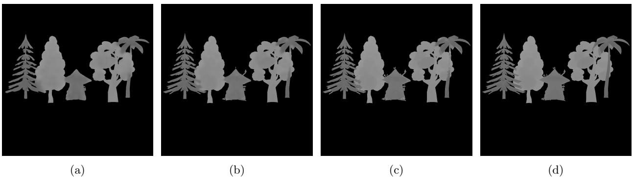
Figure 3: The intermediate results generated by the network after 1,000, 4,000, and 20,000 iterations in (a), (b), and (c), respectively, are compared to the ground truth depth map in (d). During the early iteration stages, the network converges towards a relevant solution but lacks the intricate details present in the ground truth depth map. Nevertheless, as the iteration count increases, the network gradually integrates the missing details into its predicted depth map.
