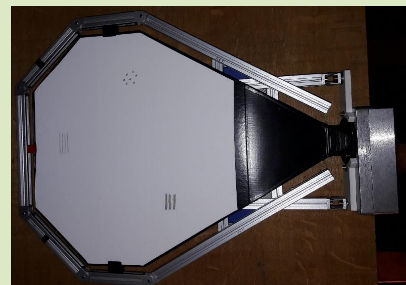
Different sizes of scratching performed on the screen. Critical size is 2 mm: if any damage is greater, the screen must be replaced.
