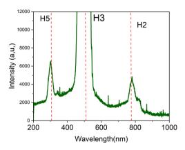
Fig. 3. Spectra emitted from MgO crystal using Ocean Optics (Maya 2000 pro) (200 nm-1200 nm)
