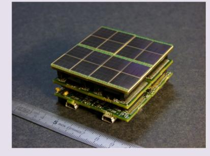
The electronic contains two 32 channels EASIROC ASICs with fully analogical front end electronics dedicated to gain trimming and readout of the **SiPMs**
