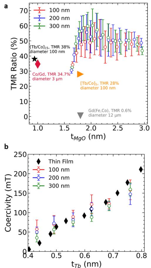
FIG. 3. a) The device average TMR versus naturally oxidized MgO thickness for nominal diameter between 100 nm to 300 nm and thicknesses  $t_{Tb}$  from 0.5 nm to 0.75 nm and  $t_{Co}=1.4$  nm, respectively compared to literature values[21, 25, 26, 39]. b) Coercive field vs Tb thickness comparison between thin film sample and nano-patterned devices.
