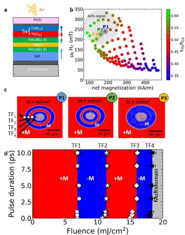
FIG. 1. a) AOS-MTJ stack with bottom-pinned and  $[\text{Tb}/\text{Co}]_N$ ML storage layer schematic. b) MOKE magnetometer measured coercive field vs net magnetization,  $M_S, \text{Co} = 760 \text{ kA/m}$ ,  $M_S, \text{Tb} = 1350 \text{ kA/m}$  [28, 29].
