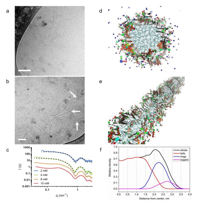
**Figure 1.** Structural characterization of SQ-Dox nanoparticles (a), (b). Cryo-TEM micrographs of SQ-Dox nanoparticles suspensions prepared at (a) 2 mM (scale bar, 50 nm) and (b) 4 mM of SQ-Dox in water. The arrows indicate the interaction sites between SQ-Dox thin cylinders (scale bar, 100 nm). (c) Small angle X-ray scattering pattern of SQ-Dox nanoparticles in water. The plain lines represent experimental data and the dotted lines are the corresponding fits. Curves are shifted
