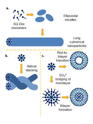
**Figure 6.** Schematic representation of the mechanisms of SQ-Dox assembly into elongated nanoparticles. (a) Early stages of assembly – spontaneous formation of short cylindrical micelles and their elongation. (b) Late stages of assembly with monovalent anions. (c) Late stages of assembly with divalent anions. Dox headgroups are shown as filled circles and squalene tails as rods. In panels (b) and (c) the hydrophobic areas are cyan while white areas are assumed to be filled with water.
