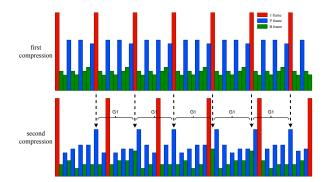
**Fig. 2**. A schematic diagram of artifacts in the prediction residuals of P-frames in a video compressed with B-frames, presented by quasi-periodic abnormal peaks. At the 2nd, 4th and 5th arrow the abnormal residual increase occurs in the subsequent P-frame of an I-B frame.
