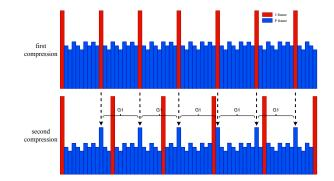
**Fig. 1**. When a video is compressed, *intra* frames (blue) are encoded independently of other frames, while *predicted* frames (red) only encode changes relative to previous frames. If the image is compressed twice, the prediction residuals of predicted frames are higher for the frames that were intra frames in the first compression than for those that were already predicted frames. This abnormal periodic peak can be detected as evidence of the double compression.
