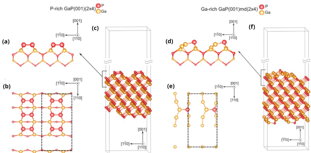
FIG. 3. (a) Side profile, (b) top view, and (c) the slab realized for P-rich GaP(001)  $(2 \times 4)$  surface. (d) Side profile, (e) top view, and (f) the slab realized for Ga-rich GaP(001)  $(2 \times 4)$ md surface. Dashed lines in the top views indicate the unit cells of the reconstructions.
