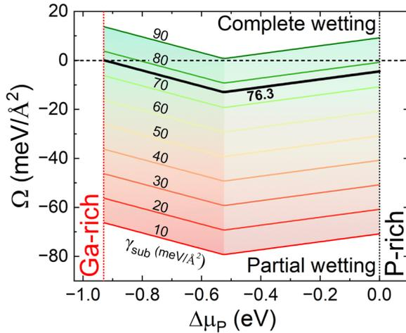
FIG. 9. Young-Dupré spreading parameter  $\Omega$  as a function of the chemical potential  $\Delta\mu_P$ , calculated for different substrate surface energies [from  $10 \text{ meV}/\text{\AA}^2$  (red) to  $90 \text{ meV}/\text{\AA}^2$  (green)], with the most stable Ga-compensated III-V/Si interface.
