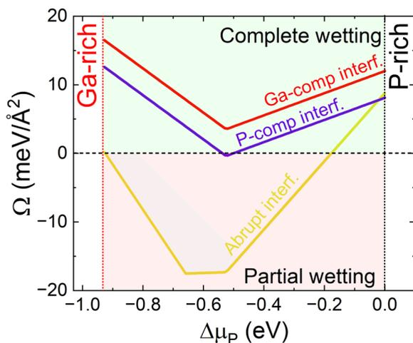
FIG. 8. Young-Dupré spreading parameter  $\Omega$  as a function of the chemical potential  $\Delta\mu_P$ , calculated for the different interface atomic configurations: (i) Abrupt III-V/Si interfaces (orange), (ii) P-compensated III-V/Si interface (purple), and (iii) Ga-compensated III-V/Si interface (red).
