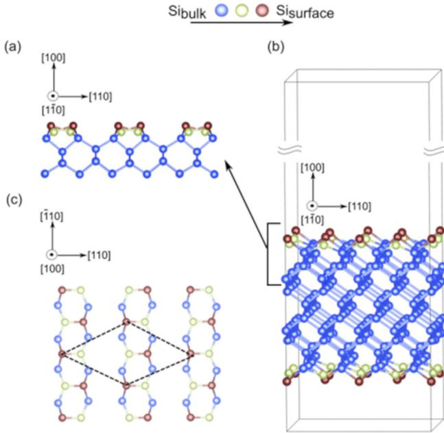
FIG. 2. The Si(001) surface studied by density functional theory (DFT) with (a) side view of the  $c(4 \times 2)$ -reconstructed surface, (b) slab with symmetric surfaces realized for DFT calculations, and (c) surface top view with the primitive cell indicated by dashed lines.
