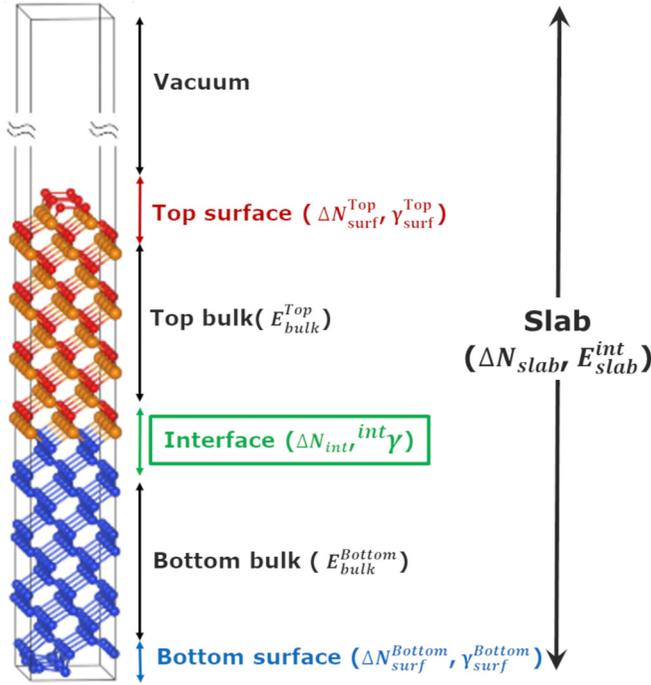
FIG. 1. Schematic of a supercell used for absolute interface energy determination, where the most important energy contributions  $E$  and  $\gamma$  are identified. Excess or lack of atoms induced by the surfaces and the interface as compared with the bulk is given by the deviation to the bulk stoichiometry  $\Delta N$ .
