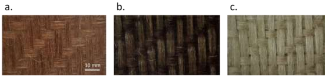
Figure 3: Evolution of the appearance of the composite specimens during hydrothermal ageing. a.) Before immersion, b.) immediately after removal from water after 50 days of hydrothermal ageing and c.) after hydrothermal ageing and drying.
