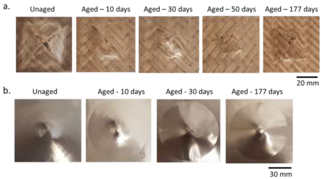
Figure 10: Back surfaces of impacted specimens after different hydrothermal ageing times. (a) composite specimens and (b) hybrid specimens.
