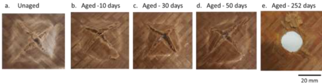
Figure 17: Back surfaces of the composite specimens after impact tests after different thermal ageing times.
