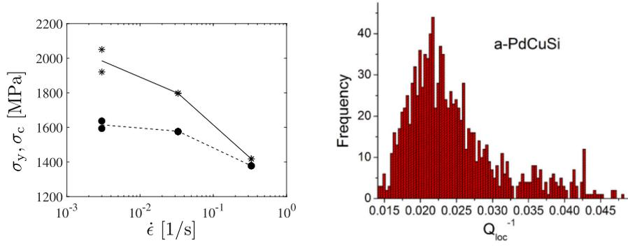
**Fig. 3.** Yield strengths  $\sigma_y$  (dashed) and  $\sigma_c$  (solid) vs. strain rate of  $\text{Zr}_{65}\text{Cu}_{15}\text{Ni}_{10}\text{Al}_{10}$  (left). The frequency of the inverse quality factor  $Q_{\text{loc}}^{-1}$  of a Pd-based BMG corresponding to the maximal frequency and representing the internal COF (Wagner et al., 2014) (right).
