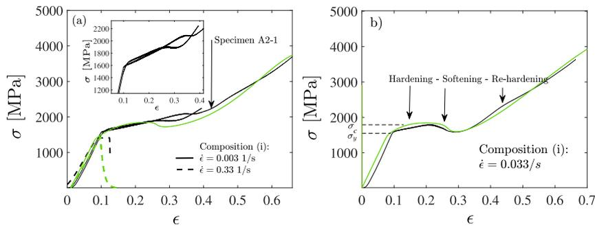
**Fig. 9.** Predicted (green) and measured (black) stress vs. strain responses of the composition (i) under the monotonic loads, when  $\dot{\epsilon} = 0.003$  /s,  $\dot{\epsilon} = 0.33$  /s (a), and  $\dot{\epsilon} = 0.033$  /s (b). The inset shows the serrated flow before the re-hardening (a).
