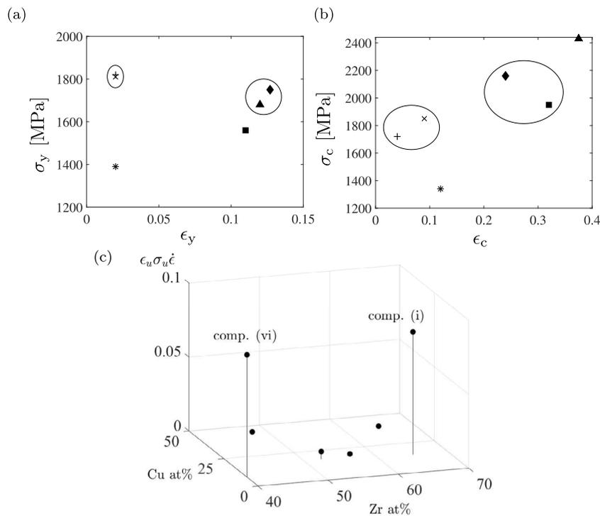
Fig. 8. A chart representing the yield strength vs. yield strain for different chemical compositions: (i) (marker ■), (ii) (marker X), (iii) (marker +), (iv) (marker \*), (v) (marker ◆), and (vi) (marker ▲) (a). Data represent mean values. Two observed clusters are highlighted by ellipses. Corresponding upper yield strengths vs. strains (b). Ductility in terms of the product  $\sigma_u \epsilon_u \dot{\epsilon}$  (c). The compositions are identified in Table 2.
