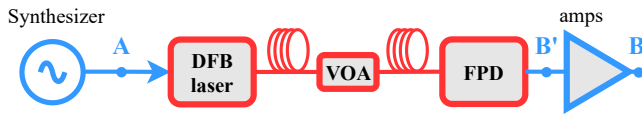
Fig. 1. Experimental set-up for basic characterizations of current-to-phase dependence. DFB: Distributed feedback laser. VOA: voltage-controlled optical attenuator. FPD: fast photodiode. The length of fiber patches is about 1 m.
