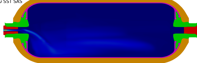
Figure 7: Scenario D10Q2. Comparison of the effective thermal diffusivity fields predicted by the k-\omega SST (upper views) and k-\omega SST SAS (lower views) turbulence models, at three time instants: (A) 200 s, (B) 400 s and (C) 600 s.
