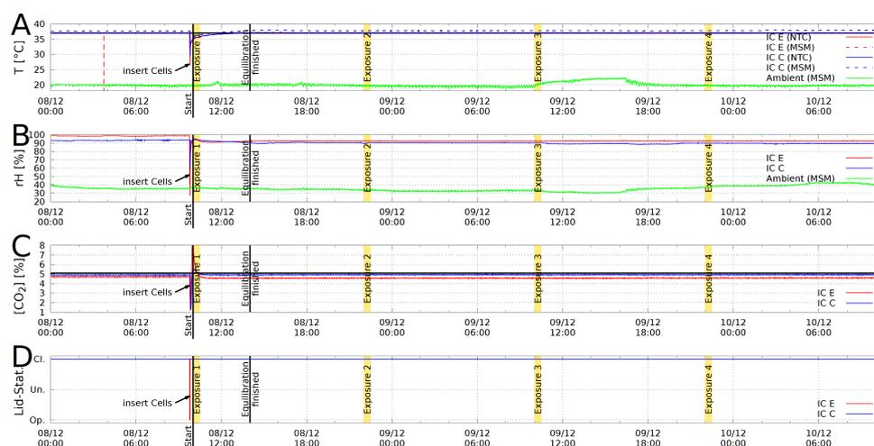
**Figure 4.** Example for a log file plot from Incubator C (blue curves) and E (red curves). (A): Temperature  $T$  in  $^{\circ}\text{C}$ ; (B): relative humidity  $rH$  in %; (C):  $\text{CO}_2$  concentration  $[\text{CO}_2]$  in %; (D): Lid status open/undefined/closed. Exposure durations are marked yellow and the ambient temperatures are represented by green lines. Double temperature measurement with negative temperature coefficient NTC sensor (solid) and a multisensor module (MSM, dashed).
