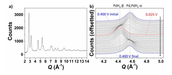
Figure 2. Time-resolved monitoring of insertion and de-insertion of H atoms into the Pd/C nanoparticles during cyclic voltammetry. a) Background subtracted WAXS pattern recorded *in*
