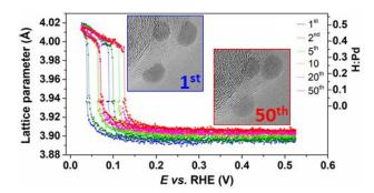
By combining *in situ* X-ray scattering and electrochemistry, we provide evidence of continuous expansion of the lattice of 3.6 nm carbon-supported Pd nanoparticles during repeated H insertion/de-insertion cycles, resulting in a progressive loss of their reversible H sorption capacity.
