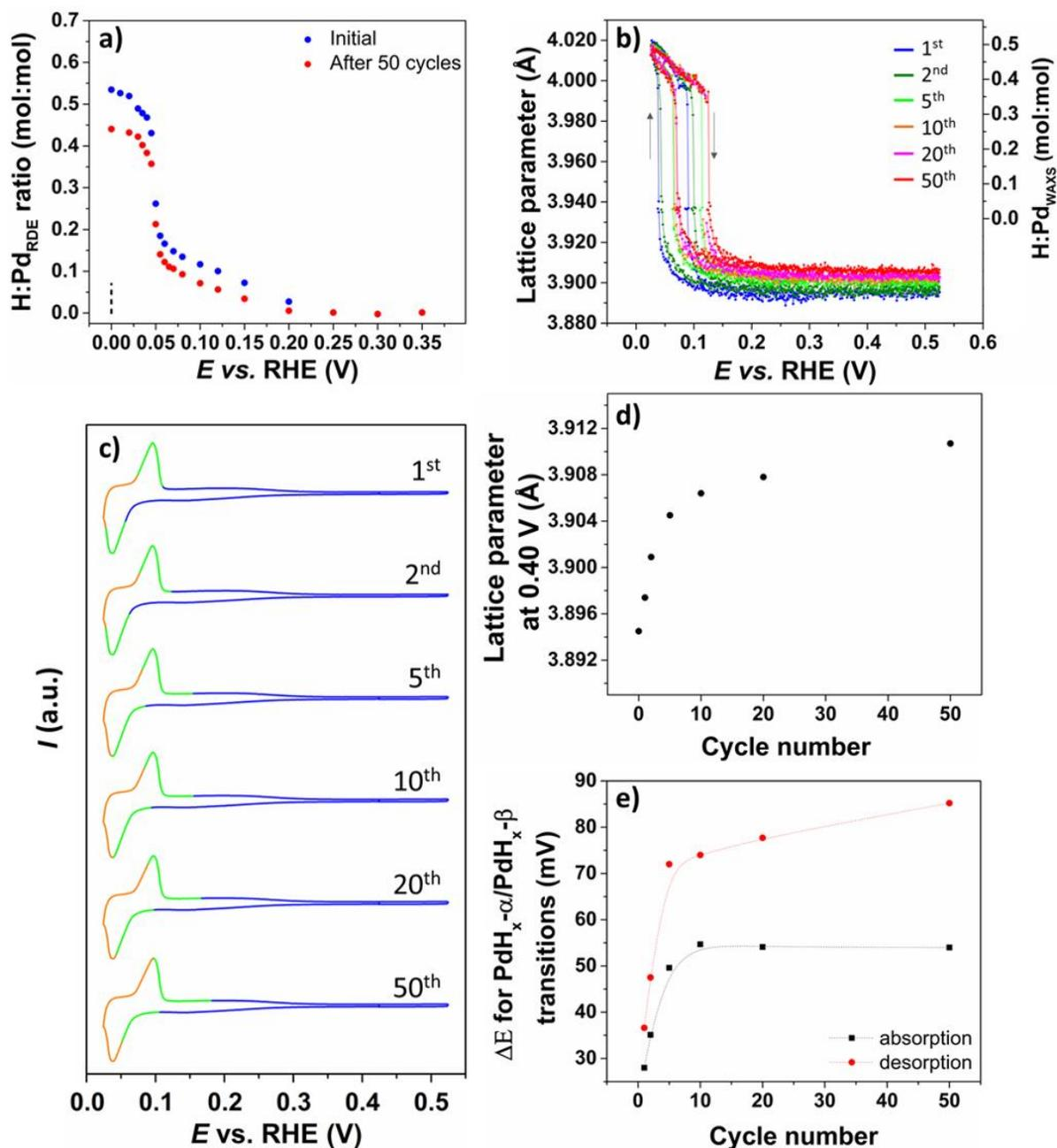
**Figure 3.** Monitoring the hydrogen-induced phase transformation of Pd/C nanoparticles *via* the combination of electrochemistry and *in situ* WAXS. (a) H:Pd<sub>RDE</sub> ratio determined by coulometric
