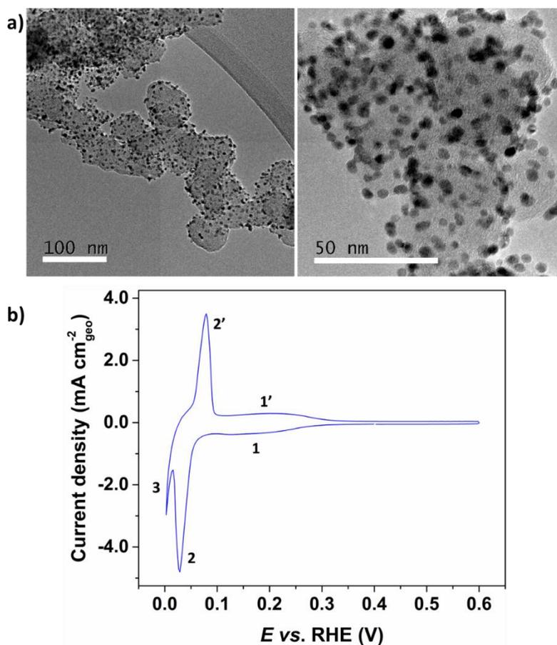
**Figure 1. Microscopic and electrochemical characterization of the Pd/C nanocatalyst used in this study.** a) Low- and medium-magnification conventional TEM images, and b) cyclic voltammograms recorded on the Pd/C catalyst in Ar-saturated 0.1 M HClO<sub>4</sub> at a potential sweep
