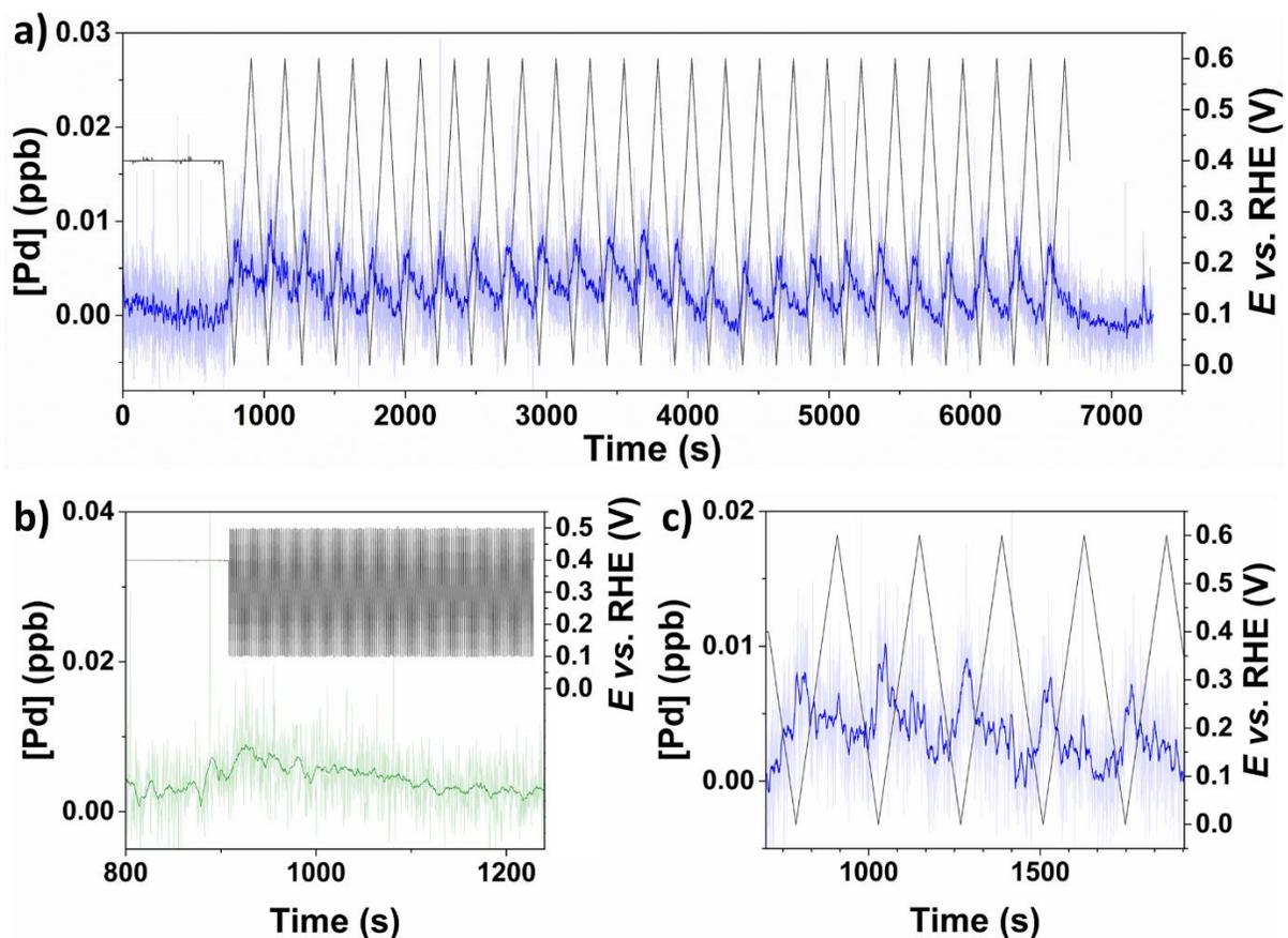
**Figure 5.** *In situ* monitoring of the amount of Pd being dissolved during successive cyclic voltammograms. a) corresponds to the cycles between 0.025 and 0.600 V and b) to the break-in. c) is a focus on the first five cycles. The blue and green lines are Savitzky-Golay averages (50 pts window) of the raw data points plotted with transparency for clarity. Ar-saturated 0.1 M HClO<sub>4</sub>,  $T = 25^{\circ}\text{C}$ .
