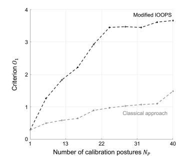
Figure 6: Comparison of the evolution of  $O_1$  criterion for the leg when OCP were calculated using the proposed modified IOOPS (black) relative to a conventional classical approach (gray).
