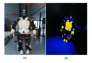
Figure 3: (a) Experimental setup and retro-reflective marker locations and (b) infra-red view of a SS camera.
