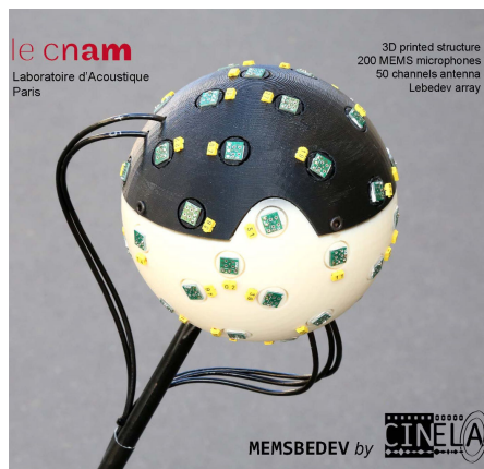
Figure 9: MemsBedeV microphone arrays with N = 50 MEMS microphones
