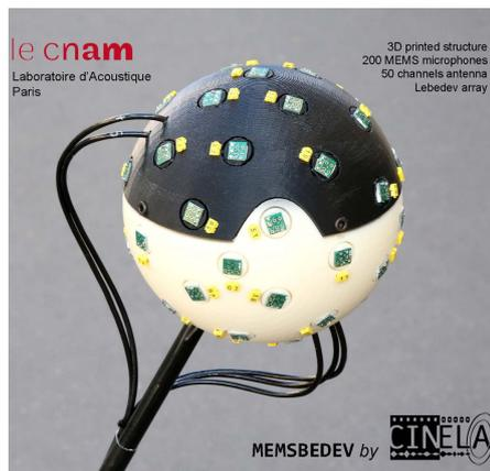
Figure 9: MemsBedeV microphone arrays with  $N = 50$  MEMS microphones
