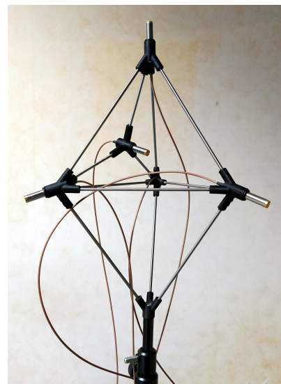
Figure 4: Prototype of an open SMA configuration with 4 B&K© 4958 microphones in a tetrahedral arrangement plus a fifth microphone pointing at the sphere center.
