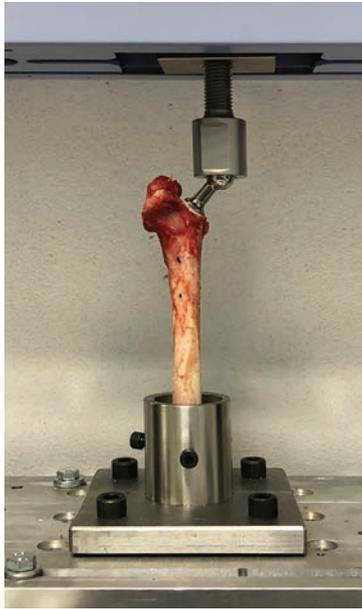
**Figure 3**—Photograph of a cadaveric canine femur after implantation of a femoral stem. The specimen has been positioned in a servohydraulic press for biomechanical testing. The base can move in all directions in the horizontal plane, permitting alignment with the manufactured cup that receives the femoral head.
