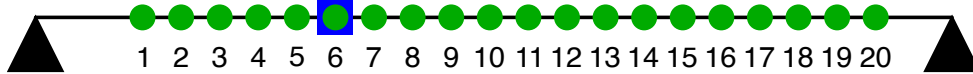
Figure 2: Location of the accelerometers and the impact location on the beam - (■) Hammer impact and (●) Accelerometers
