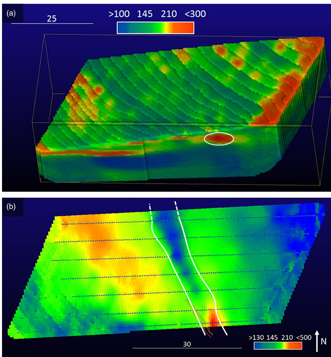
**FIGURE 6** Model pictures. The values are resistivities expressed in  $\Omega\cdot\text{m}$ . (a) Complete model with the cave entrance highlighted by a white circle and (b) plan view of the model cut at 155 m above sea level. The white outlines delimit the supposed position of the cave according to the 3D modelling.
