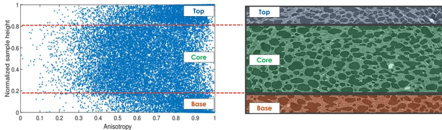
Figure 8: Relationship between sample height and anisotropy.
