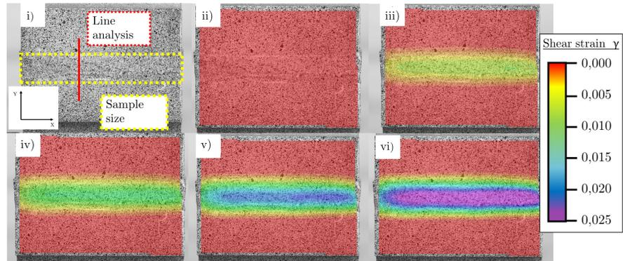
(a) Sample size on picture (i), and strain field during the test at loading = 0 %  $F_{max}$  (ii), loading = 25 %  $F_{max}$  (iii), loading = 50 %  $F_{max}$  (iv), loading = 75 %  $F_{max}$  (v), and before fracture (vi).
