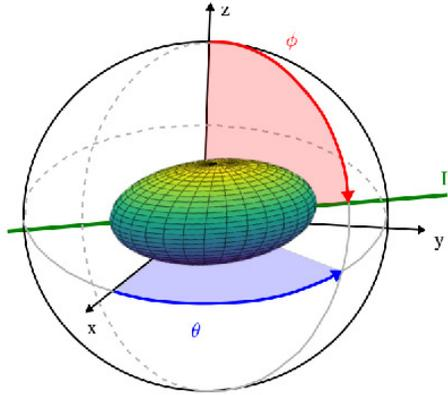
Figure 5: Orientation of the cells in a spherical coordinate system.
