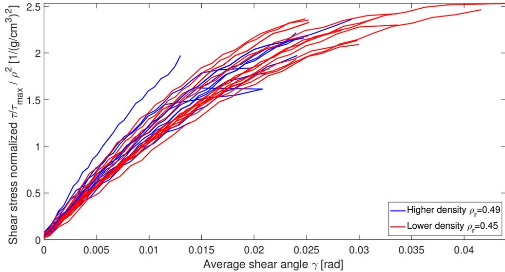
Figure 14: Stress-strain Arcan curves normalized by squared density.
