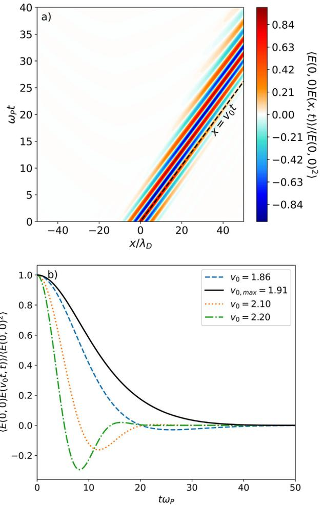
**FIG. 2.** Correlation function of the electric field with Langmuir dispersion and for a spectrum with parameters  $k_0 = 1$ ,  $\delta k = 0.4$ ,  $M = 201$ , and  $a_0 = 8.0 \times 10^{-4}$ . (a) Correlation as a function of time and distance, dashed diagonal line for  $x = v_{0,max}t$ , where  $v_{0,max}$  corresponds to the velocity where QL diffusion is maximal and (b) correlations functions at  $x = v_0 t$  for different velocities  $v_0$ .
