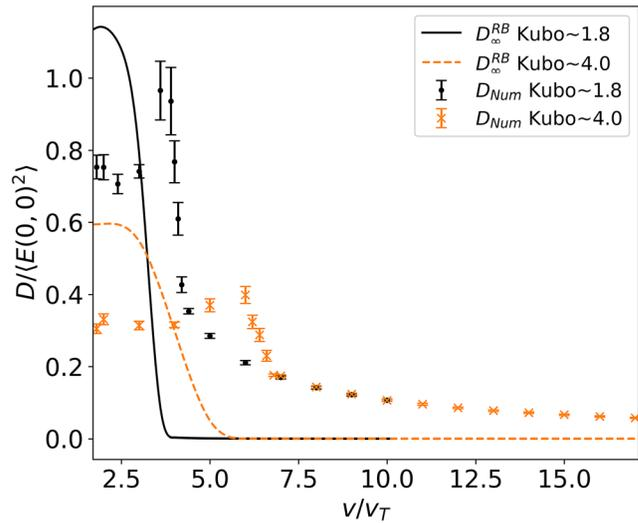
FIG. 5. Comparison of analytic (solid, dotted, and dashed lines) and numerical (points, crosses, and stars) diffusion coefficients as a function of the initial velocity of particles  $v$  for Kubo number of 1.8 and 4.0, with Langmuir dispersion relation.
