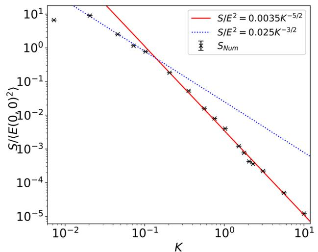
FIG. 7. Numerical  $S$  coefficient in crosses as a function of the Kubo number  $K$  after a time much larger than  $\tau_0$ , for  $v_0 = 1.95$ . The power law fit dependence on Kubo number of diffusion is in solid and dashed lines.
