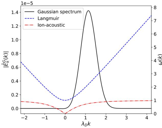
**FIG. 1.** Turbulent electric field characteristics: In solid line wave number spectrum from Eq. (17), in blue dashed line the Langmuir wave dispersion relation, and in red dash-dotted the ion-acoustic wave dispersion relation, with arbitrary amplitude  $a_0$  and parameters  $\lambda_D k_0 = 1$ ,  $\lambda_D \delta k = 0.4$ .
