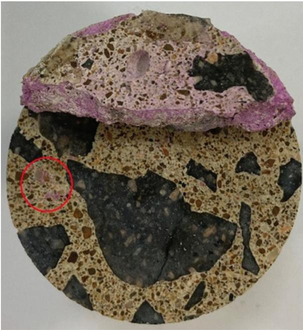
Figure 4. Specimens used for carbonation depth analysis.
