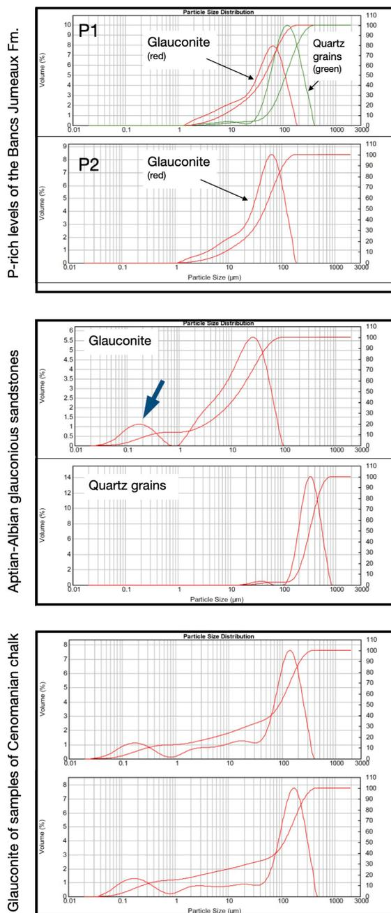
**Figure 4.** Illustrations of the grain size distribution patterns for glauconite and quartz grains of the P1 and P2 levels of the Bancs Jumeaux Fm., the Aptian-Albian sandstones and the Cenomanian chalk. The arrow points to a clay-sized fraction of glauconite probably released during grain wear induced by the measuring device.
