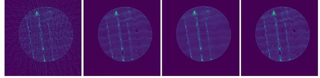
Figure 1. Illustration of natural cork samples reconstructions. From left to right : sparse and dense reconstructions then post-processing of the sparse reconstruction using only  $D_\theta$  and reconstruction using the regularized neural field  $F_\Phi$ .
